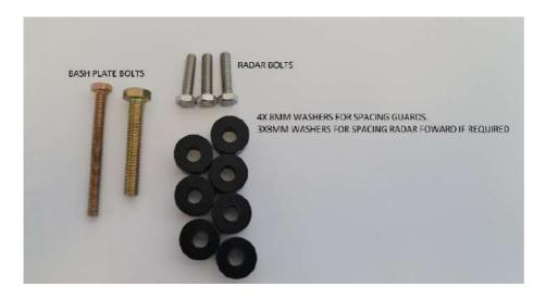
spacing guards to suit bar - each side of guard is held in with 2 bolts, remove bolts and install washer x2 each side as per below. use the longer factory bolts you removed from bumper inlieu of original bolts as they are too short.
