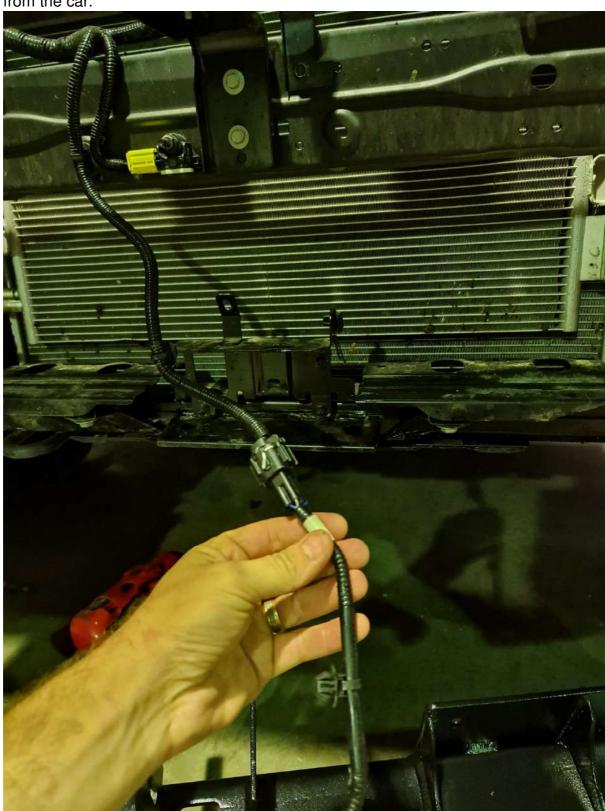
You will need take care with radar, avoid rattle gun vibration near it etc and try to keep unplugged for shortest time possible.
